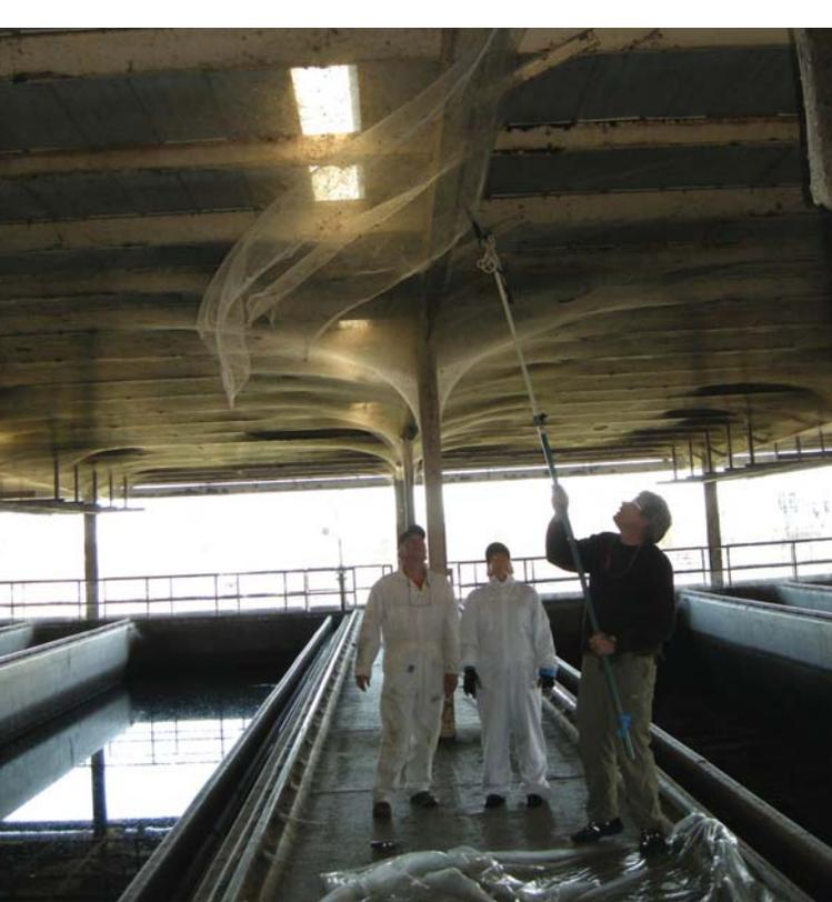
Fig. 2. Cutting sample of laminar webbing from ceiling with pole pruner saw.
