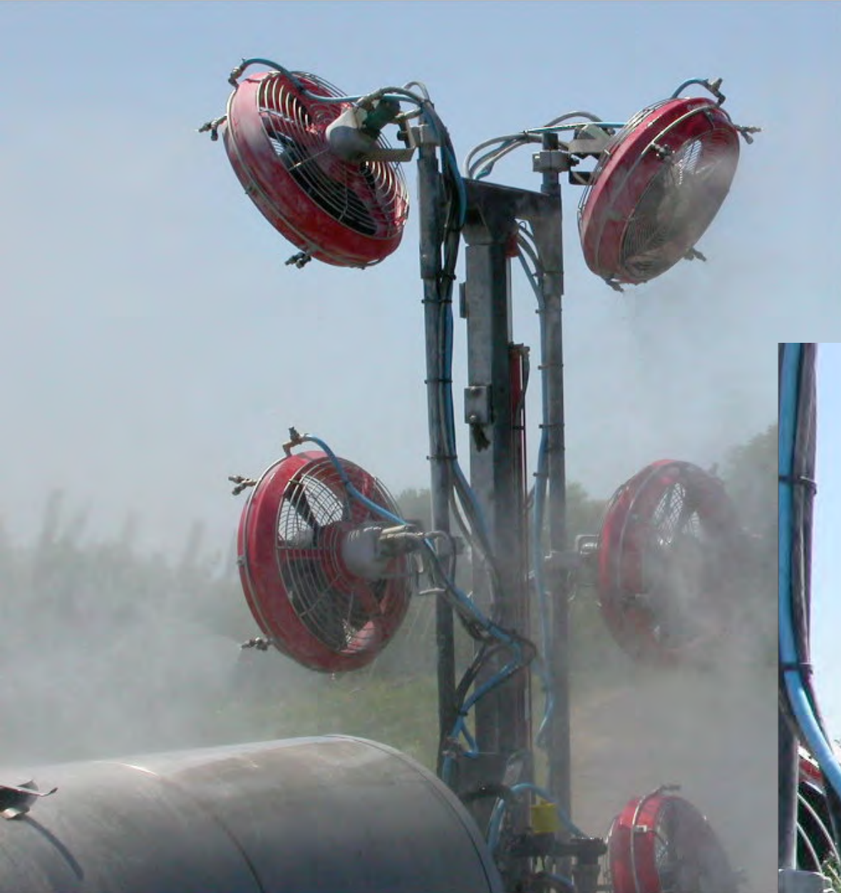
The Quantum Mist Sprayer (note that pressurized nozzles surround the fan cowling)
